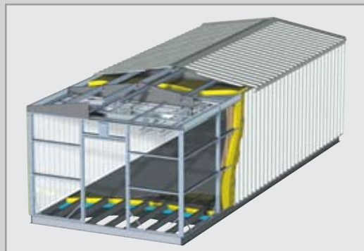
Housing structure cutaway.
