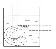
Fig. 6(b) Supply line should extend down into the sump to prevent the churning of air into the water.
