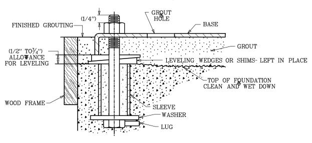
FIG. 3 TYPICAL FOUNDATION BOLT DESIGN
