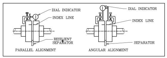
FIG. 2 TESTING ALIGNMENT, DIAL INDICATOR
