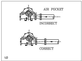
FIG. 4. SUCTION PIPING ARRANGEMENTS
