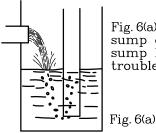
Fig. 6(a) Water falling into sump churns air into the sump liquid and causes trouble in the suction line
