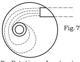
Fig. 7 Rotation of water in the well, as illustrated, can be prevented with a baffle.
